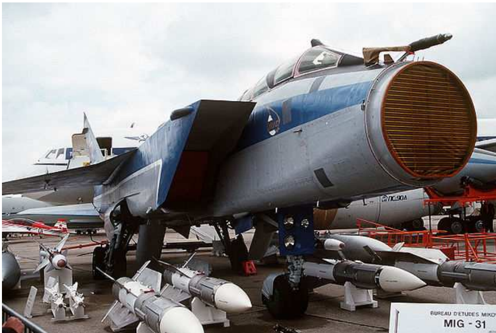
Figure 8. That orange grid under the nose cone of a fighter jet is a phased array.
